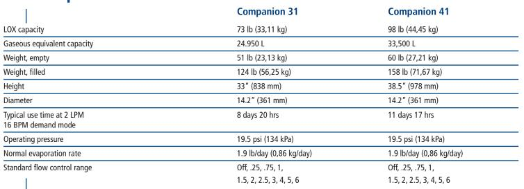
\* Standard fill times vary with the saturation and operating pressures of the source vessel. Contact Technical Service for more information.
